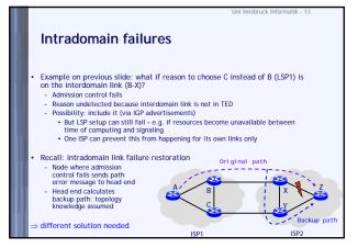
Crankback What if link X-Y does not exist or does not have enough resources? X cannot find a backup path
